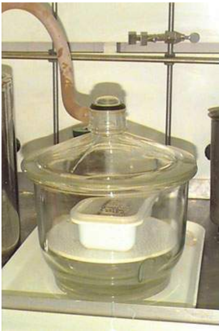
Figure 3. Shoe in vacuum chamber, housed in a container with a ventilated cap, to prevent splashing while in treatment.
