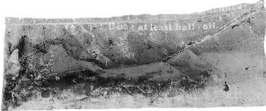
Figure 1. Waterlogged rope encased between sheets of Ziploc vegetable bag material prior to water / acetone displacement.
