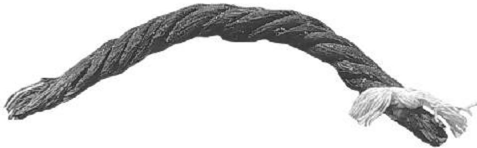
Figure 3. Silicone oil treated rope.
