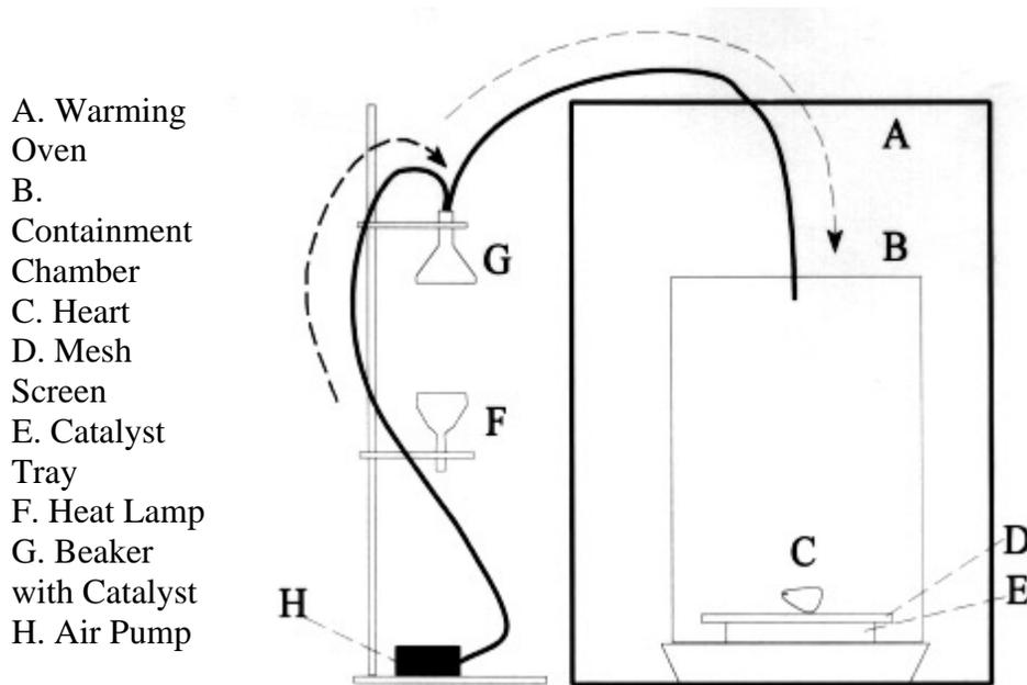
Figure 1. Set-up for polymerization of the dog heart.
