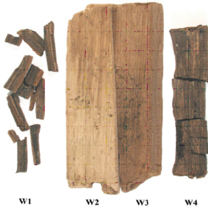
Figure 12: Group 2 wood after treatment. W1, oven dried wood; W2, MTMS treated wood; W3, Q9-1315 treated wood; W4, air-dried wood in vented fume hood. Note the comparatively lighter color of section W2.
