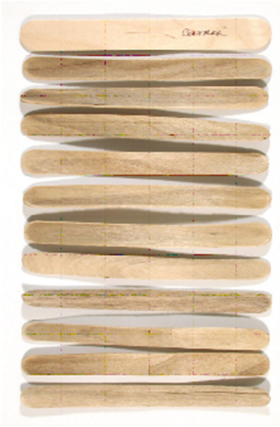
Figure 7: Control tongue depressor (top) and air-dried waterlogged tongue depressors.
