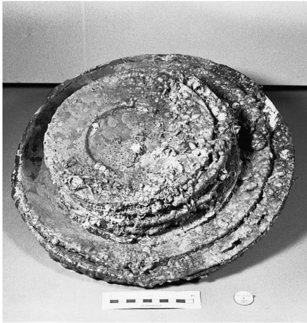
Figure 2. The stack of 22 nested pewter plates fused together by corrosion products and marine encrustation. (Photo: Jerry Livingston.)
