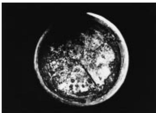
Figure 8. Back wall of the bore, showing the chaplets intersecting in the centre. (D. H. Keith)
