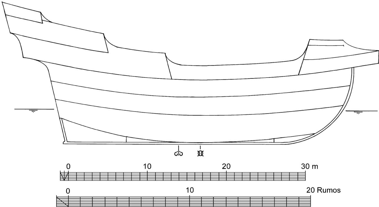
Figure 2. The Pepper Wreck as reconstructed after Fernando Oliveira’s *Livro da fabrica das naus*. (Filipe Castro)
