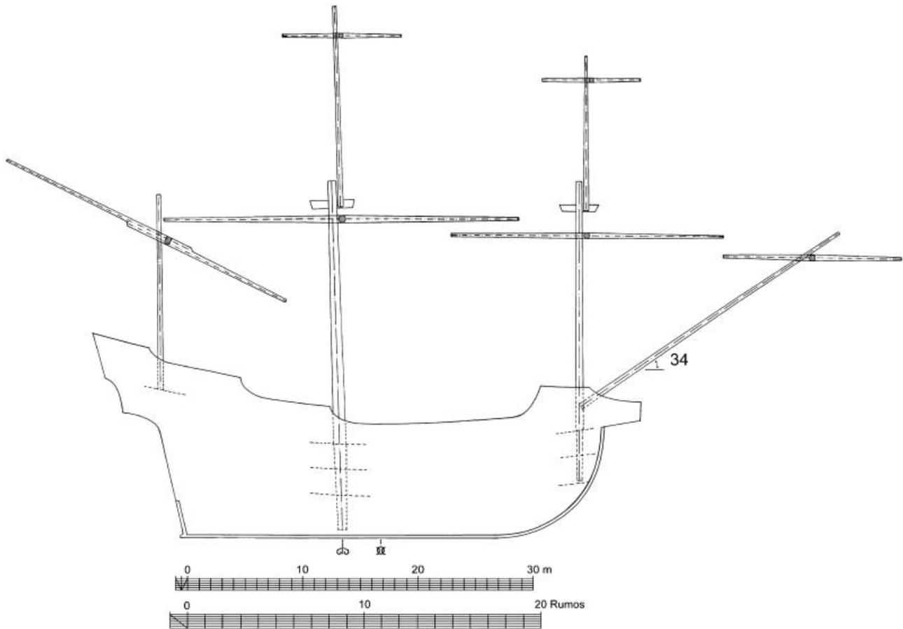
Figure 5. Plan of the Pepper Wreck masts and yards. (Filipe Castro)
